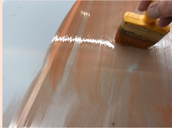
Applying the first coat of poly urethane by brush to properly fill the weave of the fabric
