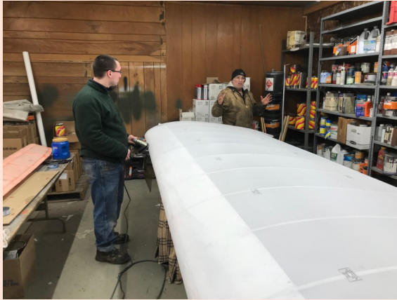
Heat shrinking the wrinkles out of the leading edge
