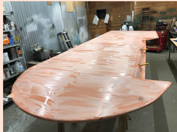
Upper full first coat complete
