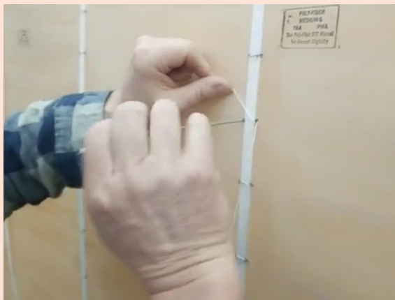
The line is pulled through the wing and returned through adjacent holes., creating a loop around the rib. The loop is secured by means of a modified seine knot
