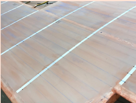
These are 1/2" tapes applied over each rib, both top and bottom of wing. This reinforces the fabric during stitching.
