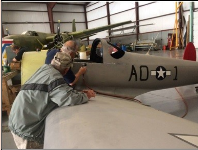
Figure 5 - riveting new sheet metal
