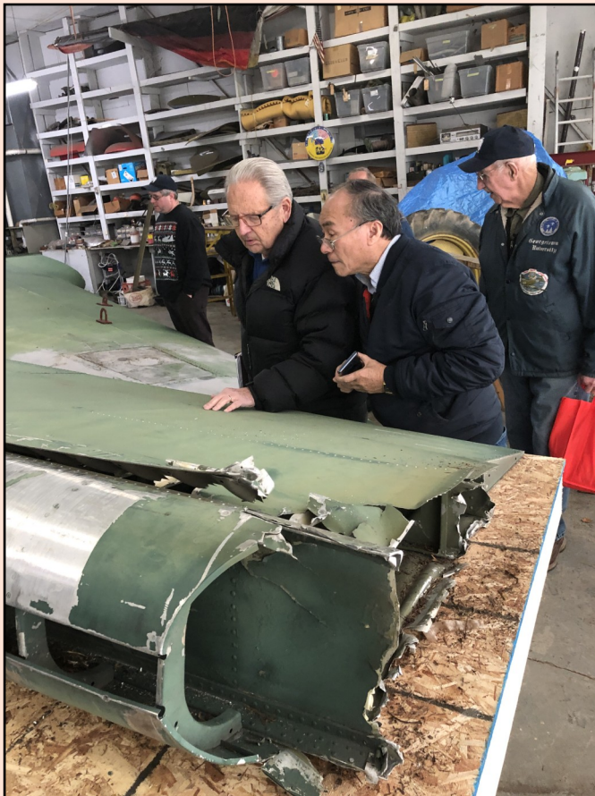
Khiem assesses the damaged rudder with volunteers Don Wilson and Ray Ingram
