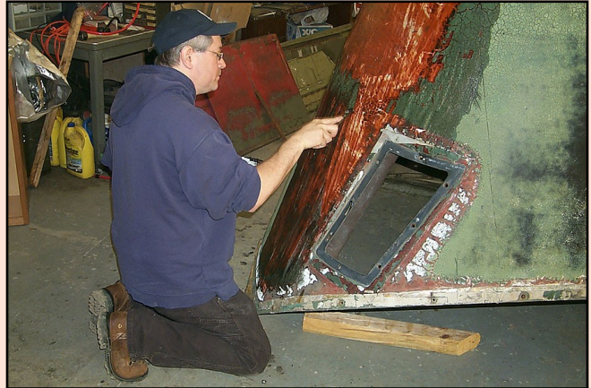
Mike Foss stripping old paint off the C130 nose. Very messy job. Intent is to coat with bed liner for protection from the elements.
