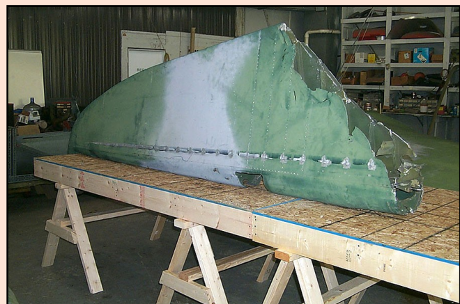
Mike Foss stripping old paint off the C130 nose. Very messy job. Intent is to coat with bed liner for protection from the elements.
