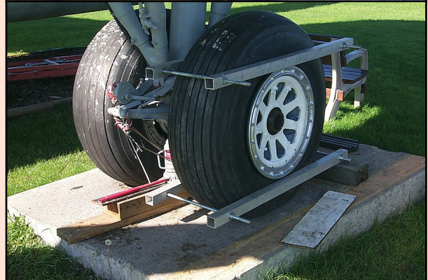
Both outside tires on the C119 gear have now been replaced. Bob Cox, Larry Jones, and Pete Bonneau worked on this.
