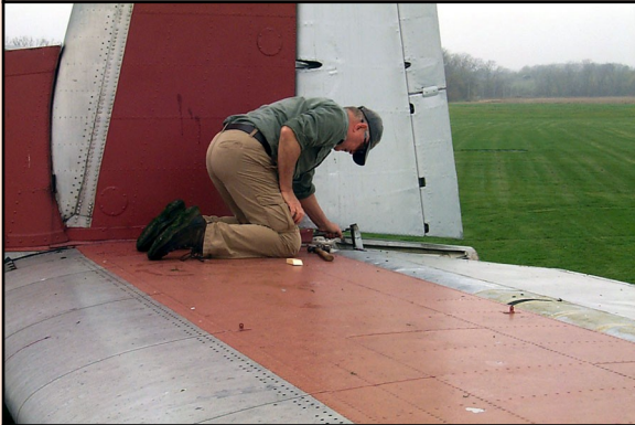
Kevin House inserted some wooden wedges into the C19 elevator to keep it stabilized until a more permanent solution can be found. We have some other repairs to make too, but will have to wait til Spring.
