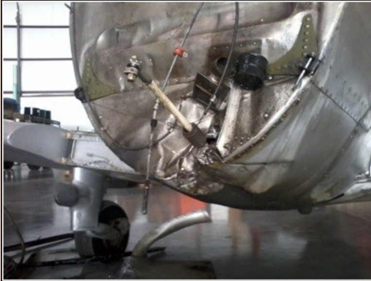
Figure 3- firewall with impression from collapsed nose gear
