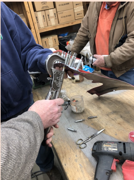
The doubler is held in place with cleco fasteners as rivets are pressed into place.
