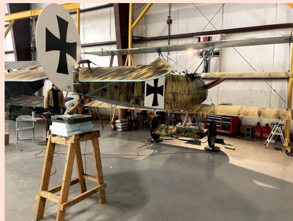
Each landing gear has a scale placed under it
