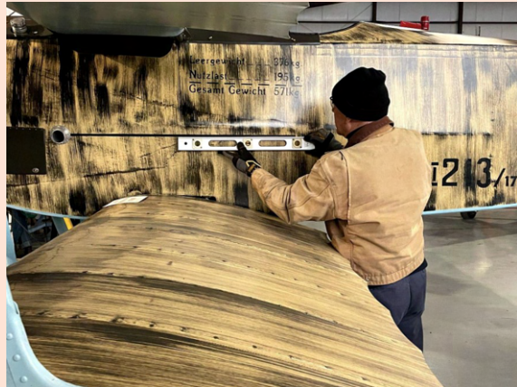
Level is checked as per the manufacturer
