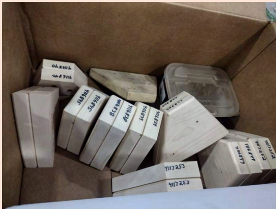
Wood forming Blocks for the intercostals
