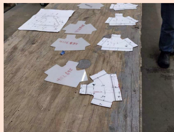
Organizing our intercostal templates. (Notice the part numbers written on each template. This will be important throughout the process!)
