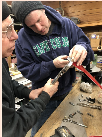
These rivets are squeezed into place. They are not "pop" rivets.
