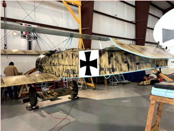
The airplane is leveled as per design
