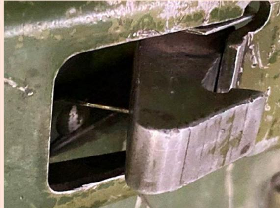
The above photos show one of the three clamshell latches of which two need spring safety latch repairs. You can see one of the broken springs circled above. They help keep the clamshell doors from accidentally opening up.
