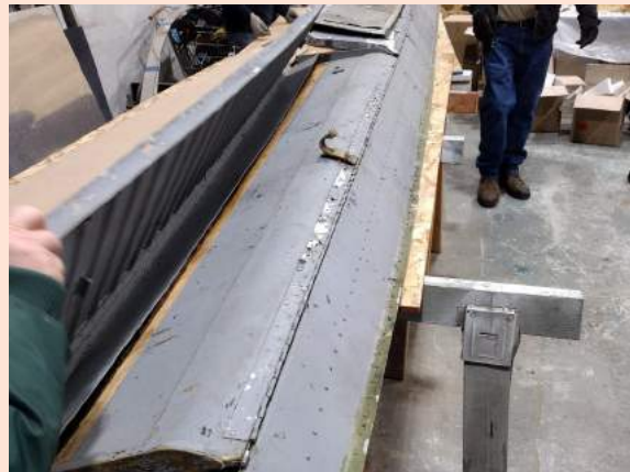
They could be folded up while inside the airplane in the event they were used for carrying cargo instead of paratroopers.
