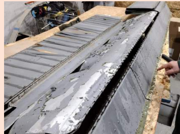
A few long pieces of small rod removed, and the sections come apart.
