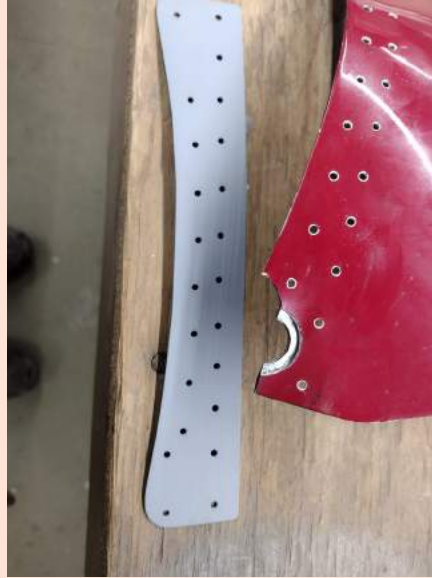
Doubler plate that was riveted to the cowling.
