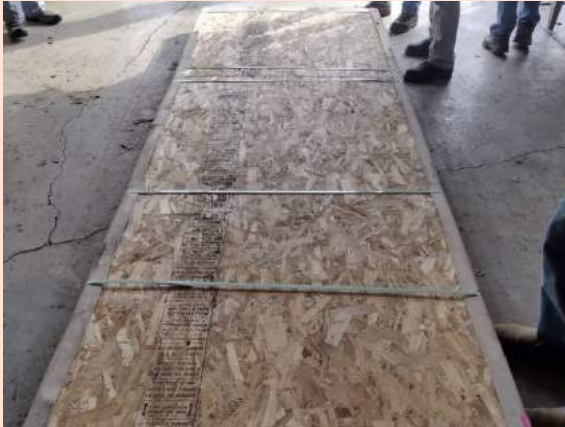
Aluminum sheets sandwiched between plywood keeps them sturdy, so they won't bend .
