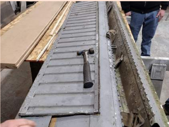
Piano hinge is used to attach the front sections to the pan seat, and to attach the pan seat to the mount that is attached to the inside of the fuselage.
