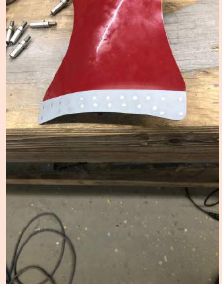
The doubler is in place and ready for painting
